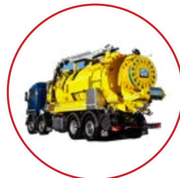
Vehicles equipped for water jetting
